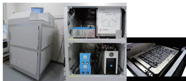
Fig. 4. Amyloid-burst inducer HANABI. Left: outside view; middle: ultrasonicator; right: microplate.
