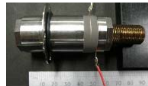
Fig. 3 Photograph of fabricated ultrasonic torsional transducer
