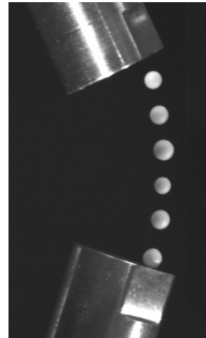
Figure 3. Trapped polystyrene particles.
