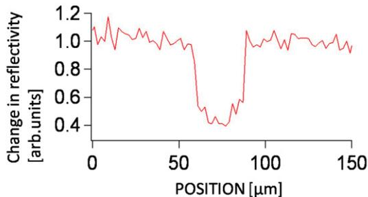
Fig.3 Normalized change of reflectivity vs. the radial position of the surface of contact area at 1 N load.
