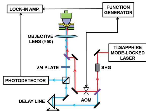
Fig. 2 Optics. AOM: acousto-optic modulator, SHG: second harmonic generation crystal
