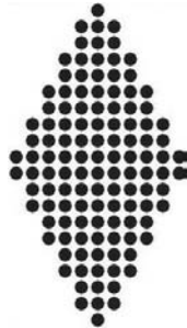
Fig. 2: An acoustic lens made of acrylic resin cylinders in air with a [100]-directional square alignment.
