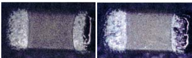
Fig.1 Surface view of multi-layer ceramic capacitors: a) non-defective specimen b) defective specimen.
